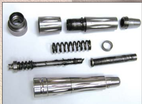
Figure 1. A popular lube-free, low-speed assembled nose cone (bottom) and disassembled nose cone parts showing extensive dirt and debris prior to cleaning and repair.
