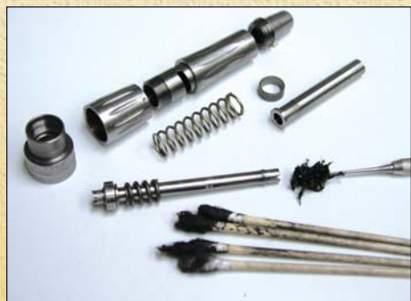
Figure 2. Disassembled nose cone post repair and cleaning. Note the residual plastic barrier pieces on the explorer tip and the internal dirt and debris removed by the cotton swabs.
