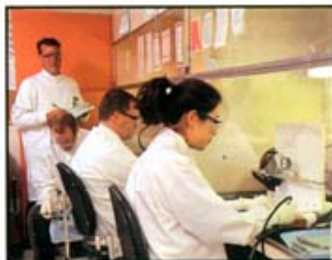
This team is testing the ability of handpieces to withstand routine heat sterilization. CRA has performed over 300,000 handpiece tests since 1990 to identify handpieces that cannot withstand the process.
