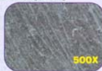
SEM image of composite resin surface polished with pumice paste. Similar scratches are evident with all brands tested.
